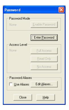
The controls within the Password Aliases group box are enabled only when either FasTrak Security or NT Authentication Security are in use. When these controls are clicked, a valid security administrator password must be entered.
