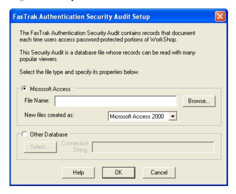
To write the local security log to a Microsoft Access database file, click the **Microsoft Access** radio button. Type the name of the Access file in the **File Name** text box or click **Browse** to locate the file. Select the proper file format from the **New files created as** group box.
