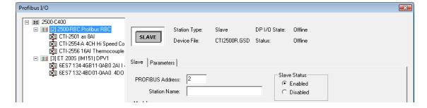
The slave devices in the Network Tree are listed in descending order of Profibus Address. Changing the Profibus Address in the **Slave** tab will reorder the devices in the Network Tree to retain descending order of address.
