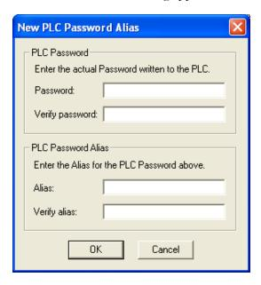
1. In the **PLC Password** area, enter the actual PLC password in the **Password** box. Verify the password by entering it again in the **Verify password** box.
