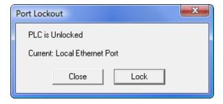
2. If the PLC is unlocked, click **Lock** to lock the communication port. The message "Lock communication ports?" appears.
