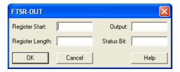
• **Register Start** - the starting address for the shift register. The four words (Register Start through Register Start + 3) are automatically reserved for the operation of the statement and make up the header of the shift register. Valid descriptors are writeable integer addresses (writeable addresses containing an integer value such as V101 or WY11).
