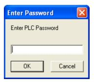
This PLC password is actually stored in the PLC. Therefore, programming packages other than 505 WorkShop also request the same PLC password when attaching to the PLC.
