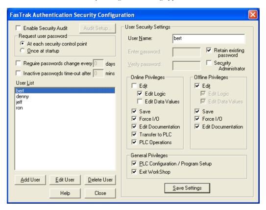
In addition to controlling user access, this security mode also can record each attempt to access protected portions of WorkShop made by users. To enable this, click the **Enable Security Audit** check box and the **Audit Setup** button.
